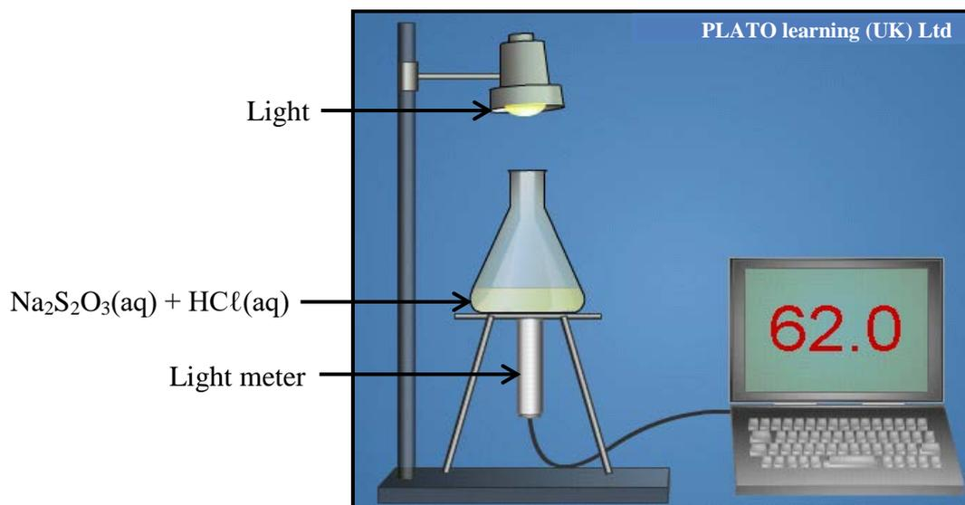
Luke uses the apparatus shown in the diagram to conduct a series of experiments to determine the relationship between the concentration of the sodium thiosulphate solution and the time taken for the light meter to show a reading of 62 lumens. (Lumens = unit for light intensity.)
